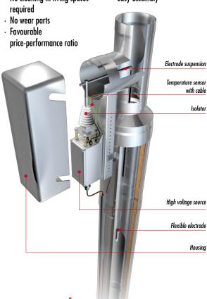
By means of a high voltage probe, electrons direct the rising dust particles towards the chimney wall. There, the fine dust deposits in the form of coarse soot and is removed by the chimney sweep during the next cleaning operation.
